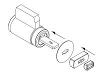
Reinstall Cylinder as Shown
